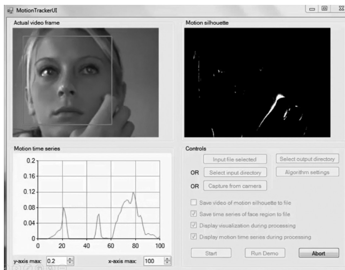
Figure 10.3. Automatic tracking of body movement from video using motion silhouettes. The image on the right displays the areas of movement from the video playing on the left. The graph on the bottom shows the amount of movement over time.
